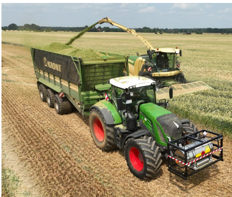
Image: Converted Fendt 936 of the RUHE Group with Bio-LNG front tank
